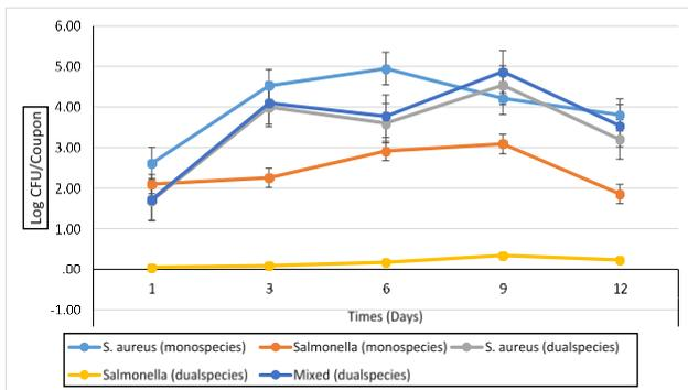
**Fig. 3:** Showing the average development of biofilm (log CFU/coupon) on galvanized steel coupons by strains of *S. typhimurium* and *S. aureus*, either mono- or dual-species, under dry conditions after a 12-day incubation period at 28°C.
