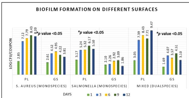
**Fig. 4:** Showing the development of biofilm (log CFU/coupon) that *S. typhimurium* and *S. aureus* strains under either mono- or dual-species conditions were able to produce on PL and GS coupons after 12 days of incubation at 28°C.
